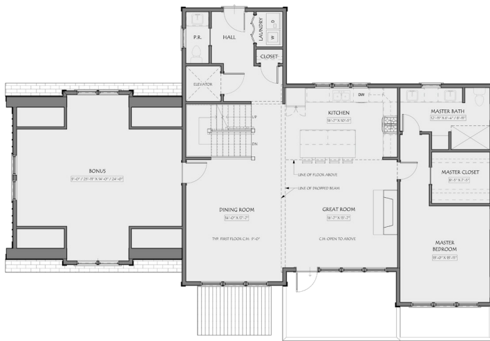
◀ FIRST FLOOR PLAN First Floor Finished Space — 1,940 s.f. Garage — 670 s.f. (basement level)
